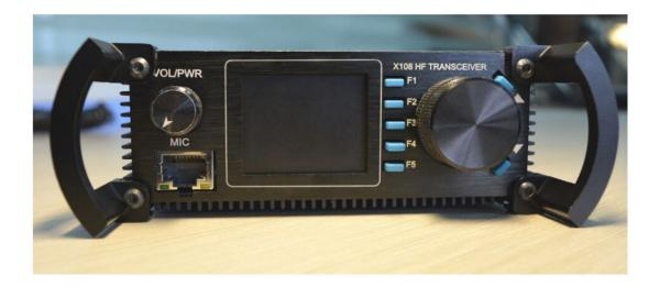
The brand new X108 from Chongqing Xiegu Technology is a compact single conversion HF transceiver covering 0.5 to 30 MHz. Boasting the latest in minimalist industrial design, it offers radio amateurs high quality HF capability at a very affordable price.
