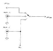
antenna's, such as an active whip, or loops. As you can see in the schematic, one of the antenna lines is phantom powered.
