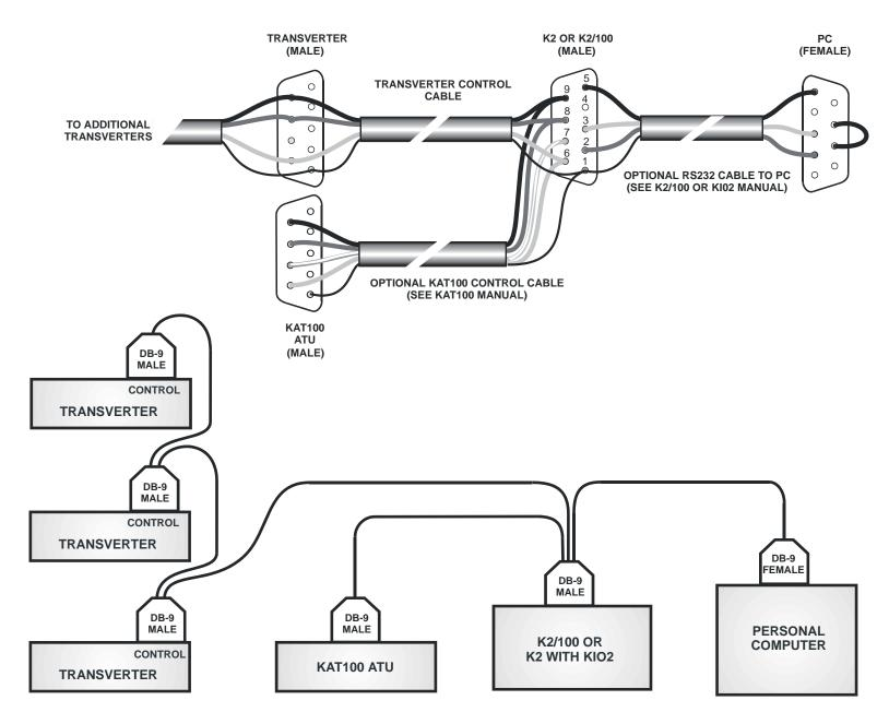
Figure 7. K2 Extended Control Cabling Hookup Diagram.
