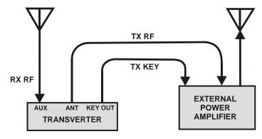
Figure 10. Using an External Power Amplifier.
