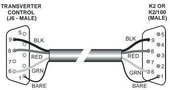
Figure 5. K2 Control Cable Wiring.
