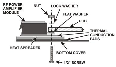
Figure 11. RF Module Mounting Hardware.
