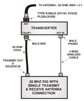
Figure 4. Connecting the Transverter to a Non-Elecraft 28-MHz Rig with a Single Transmit and Receive RF Path.
