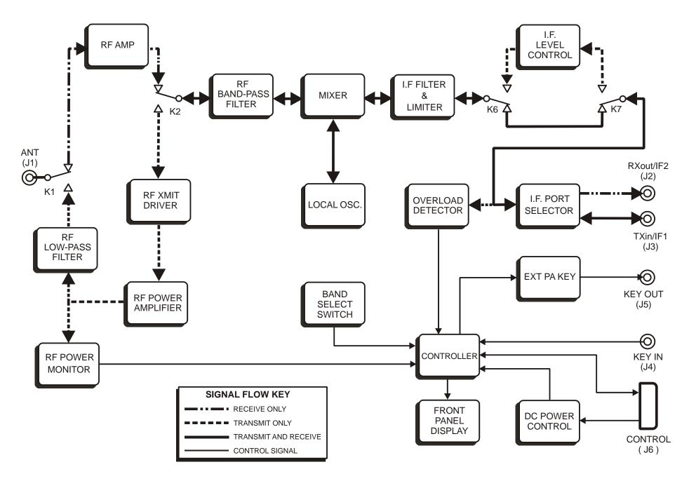
Figure 12. Transverter Block Diagram.
