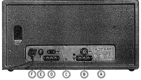
G 209-R - Rear connections. A = antenna input for coaxial cable. B = antenna input for balanced line. C = connection for stand-by remote control. D = AF output terminals (impedance: 1-2 = 3,2 ohm; 1-3 = 500 ohm). E = fuse (calibrated 2 A). F = voltage line adjustment switch.
