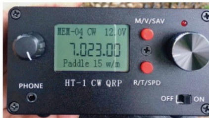
The front view of the HT-1A compact 20/40m dual band CW QRP transceiver.
