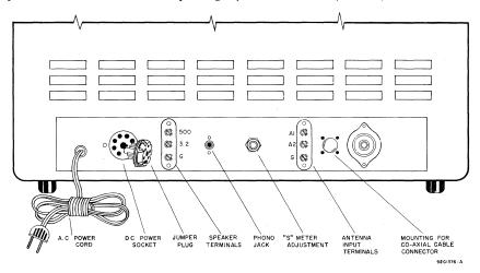
Fig. 4. Rear View of Receiver
