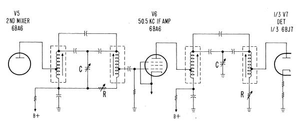
Fig. 13. Equivalent Schematic Diagram of 50.5 KC IF System
