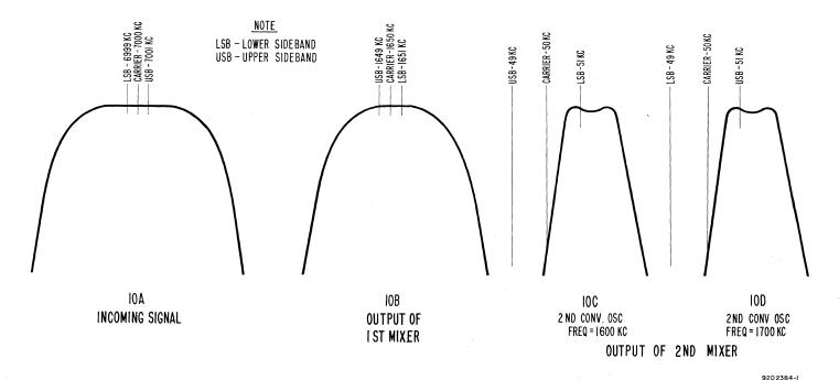
Fig. 10. Selectable-Sideband Response Curves
