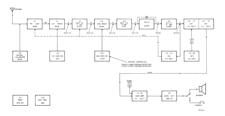
Fig. 16. Block Diagram of Receiver
