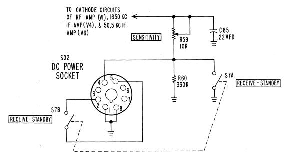
Fig. 6. Schematic Diagram of Sensitivity and Receive-Standby Circuits
