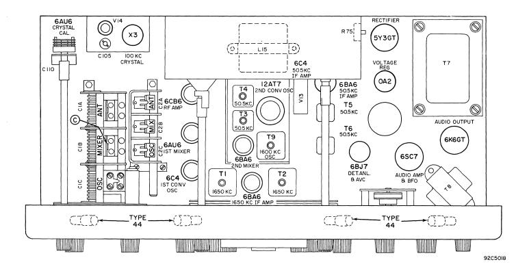
Fig. 11. Top View of Chassis Showing Location of Alignment Adjustments, Tubes, and Dial Lamps
