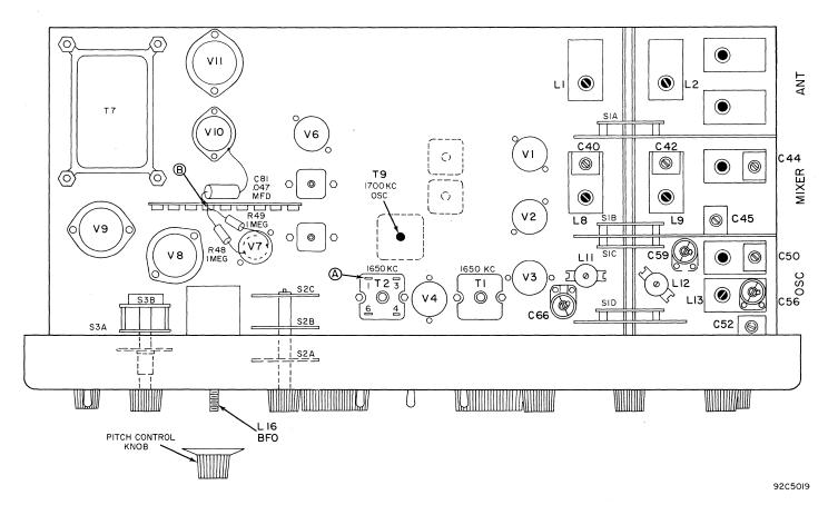
Fig. 12. Bottom View of Chassis Showing Location of Alignment Adjustments and Tubes
