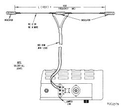
Fig. 3. Doublet Antenna Using
