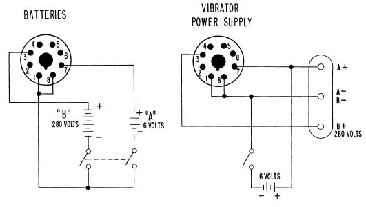
Fig. 5. Wiring Diagram for DC Operation
