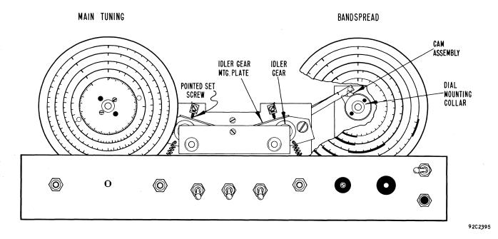
Fig. 15. Front View of Gear Drive Tuning Mechanism
