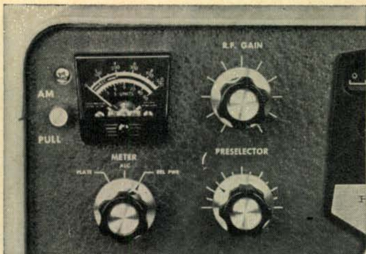
Front view of the top left corner of the SB-110. The new push-pull control can be seen to the left of the meter. The matching knob is Heathkit part No. 462-175. Decals add the finishing touch.
