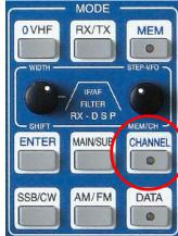
Recalling of VFO adjustments (frequency, mode and filter bandwidth) is done pushing the CHANNEL button located in the cluster MODE. It gives access to 3 banks of memory each storing 99 channels provided by PT-8000A.
