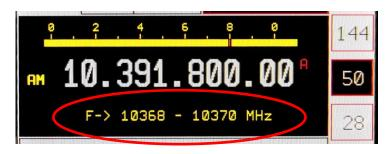
Using control STEP-VFO / MEM/CH gives access to all transverter operation frequency bands as listed below (Table 15).
