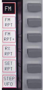
Frequency Modulation (standard mode); the softkey will be displayed inverse (as shown here); the display will show [FM] (left of frequency).
