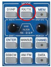
Pushing the button RX/TX located in the cluster MODE will call up two types of menus which gives access to various basic settings for RX and TX.
