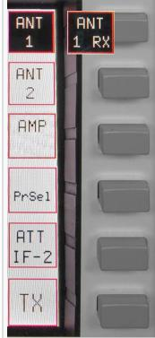
Select antenna #1 or – second press – antenna #1 for TX and an additional RX antenna; the display will show ANT 1 or ANT 1 RX if appropriate. (see Page 14, Table 10, No. 4), the softkey will display as well (inverse as shown).
