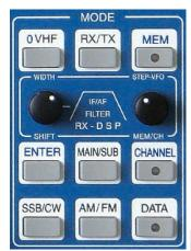
Pushing MEM button located in the cluster MODE will store the frequency and additional VFO values of the active RX to one of the 297 memory channels organized in three banks with 99 memory channels each bank.
