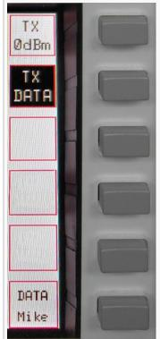
In case this softkey is activated (the softkey will be displayed inverse; DATA-LED will turn on) the signal at the OdBm input (MIC-PTT Pin 4) will be transmitted when PTT is switched.
