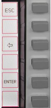
Numerical input will be aborted; the last used frequency will be displayed instead; the last used softkey menu will be called up.
