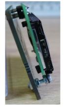
If the space available for the module integration is a bit short the depth of the sandwich may be reduced by 5-7 mm by directly soldering the LCD to the board, instead of using male and female headers. Please notice that if board removal is needed in the future, you will have to unsolder all pins from the LCD or the board.
