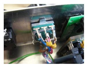
Solder two 100 nF capacitors directly to the encoder pins (between active pins and ground).
