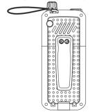
Remove hand-held mic cover:Loosen the screw by rotating, and then remove the cover.
