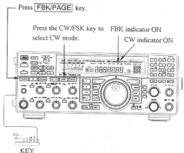
Figure 6.7 Full Break-In Operation
