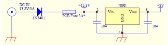
[ ] Solder 1x DC IN socket, and trim the pins flush to avoid shorts with chassis foot screws [ ] Solder 1x speaker connector near the DC IN power connector; make sure you install it in place [ ] Bend the pins of 1x 1N5401 diodes as shown, and solder. For other diodes, always bend the pins like this. If you kit comes with 1N5820~1N5822, it is an upgrade for lower dropout voltage.
