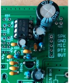
[ ] Plug in a  $12\sim13.8$  V power supply and connect an external speaker of  $8~\Omega$  or higher impedance to the speaker connector. Touch pin 5 of the nearby NE602A using tweezers to inject some noise, and note if the audio amplifier works. If not, please check your soldering, and check the pin 2 of the TDA2822M for the presence of 8V. If all is okay, disconnect the power supply and the external speaker to proceed to the next step.
