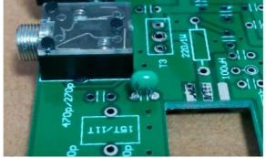
[ ] Solder the remaining parts, with the exception of all toroid coils, and the D882 and IRF530 transistors, which will be installed later in final assembly stages. When finished, it will look like the photo below.
