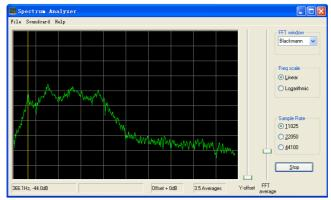
Remove the audio cable and connect an external speaker. Use band noise or a signal to peak again the RX BPF.
