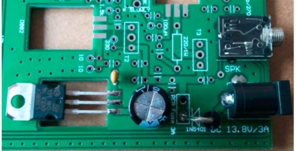
[ ] Plug in a 12~13.8 V power supply to the DC IN connector (center positive) and measure the voltage on pin 3 of 7808 near to the 104 capacitor to see if it is within +/-5 % of 8 V; if not, check power supply polarity and your soldering
