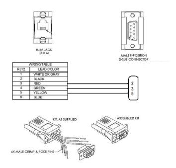
Figure 3 RJ12 (6x6) to DB9 Connection
