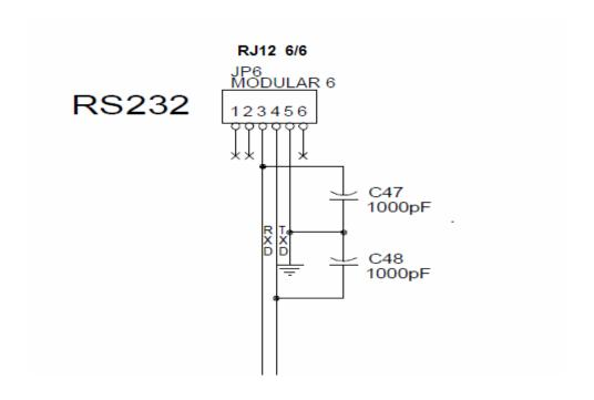
Figure 2 Kachina 505 - RJ6 Internal Wiring
