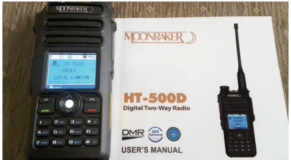
The HT 500D dual band DMR / analogue handheld and its user manual.
