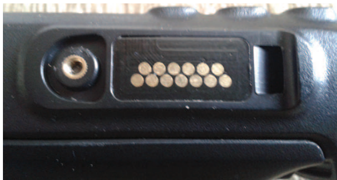
Keep the cover over this connector unless you are programming the radio.
