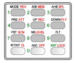
MODE REV – Short press selects between CW and SSB modes; Long press enters reverse mode – CW to CW-R or LSB to USB
