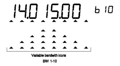
Rotating encoder 1 selects various filters from b1 to b10. Also chevron symbols just bellow operating frequency depicts relatively used bandwith.
