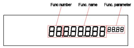
Function selection is controlled by encoder 3 or UP REC and DOWN PLY buttons. Parameter selection is controlled by encoder 4
