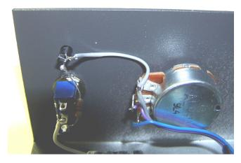
Connect the supplied 4.7K resistor to the \*switched\* 12V power on the T/R switch.
