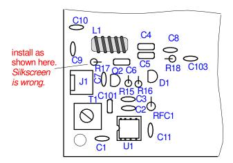
(When these components have been installed, the receiver portion of the transceiver is complete.)
