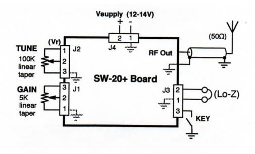
Wire the connectors and controls to the SW-20+ as shown pictorially below. Note that the keying return line lacks its own distinct board connection. This return line is shared with the headphones' return.
