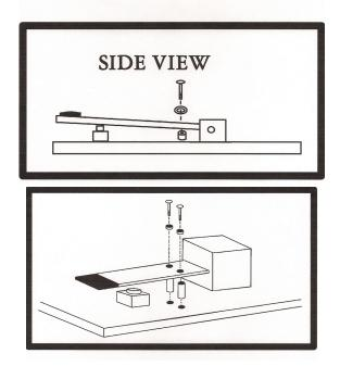
Mount the circuit board to the breadboard with four 1/2 inch brass wood screws and black 3/8th inch plastic spacers. You should have starter holes on the breadboard (Breadboard step 4.) You may need to loosen or remove the key to get the front right screw in.
