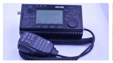
Double conversion superheterodyne + digital baseband processing , the advanced digital processing unit makes the signal clearer.
