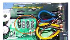
Jumpers on main board behind microphone socket
