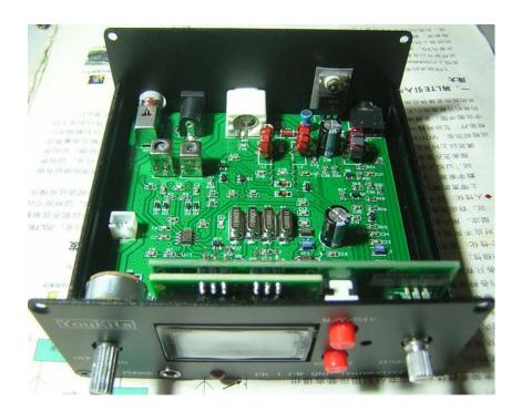
Secure the back cover with screws, put studs on the display board and then secure the front cover. Install two knobs, assemble finished.
