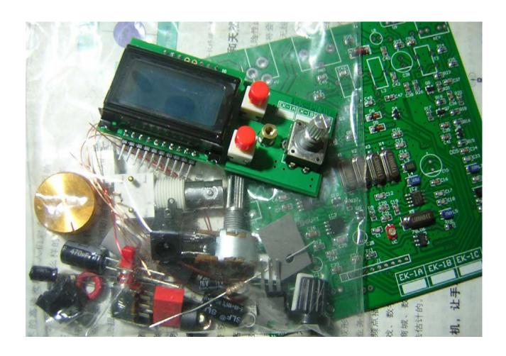
EK-1A 2014 3 Band (40m, 30m,20m) CW QRP transceiver kit is easy to build, it has SMD finished by the factory. There are 2pcs of PCB, the main board and display board. To guarantee the building success, the display board and main board have been assembled and tested including the MCU, LCD and DDS.
