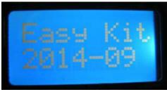
2. Waiting for 2 second, display change to below. Put your frequency counter to DDS testing point, the pad close to R27.
