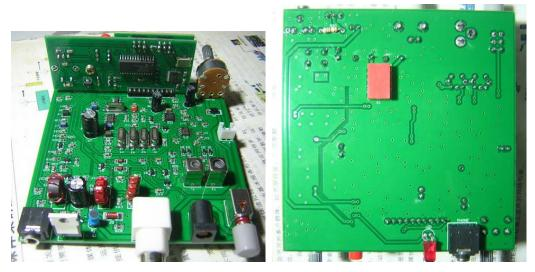
2. K1, LED, R30, PHONE are all installed at back side of PCB, please check below pic.
