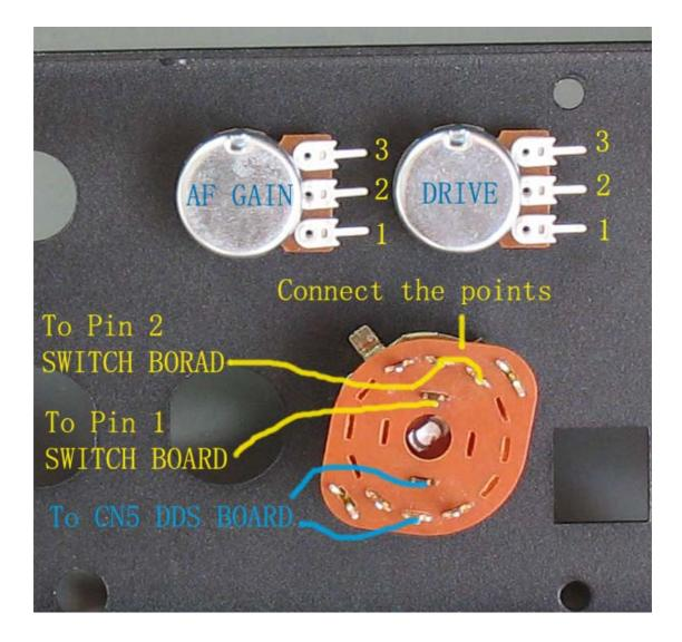
Connect the AF gain pot leads to CN3 as the number indicated. DRIVE pot is also connected the same way. Number 3 pin is connected to the GND pad.
