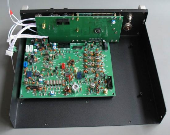
First, place the DDS assembly. Fasten it with flat screws.
