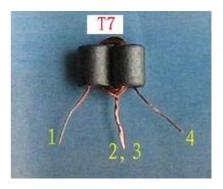
L1: 23 turns on T37-2 core. Cut 30 cm length of 0.31enameled wire for the winding, leaving about 1 cm for each lead.
