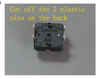
so that the keys project through the key openings with suitable clearance on all sides.
