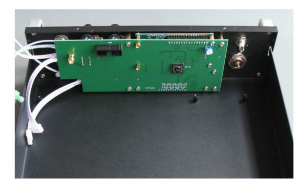
Place the main board. Use 4 screws to fasten it to the case.
