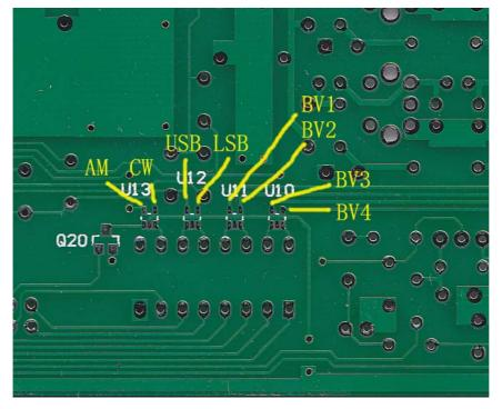
However, the voltages can be measured on the top side:
