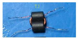
is the exact length for 9 turns with about 1 cm on each end. Wind primary first. Remove about 5
