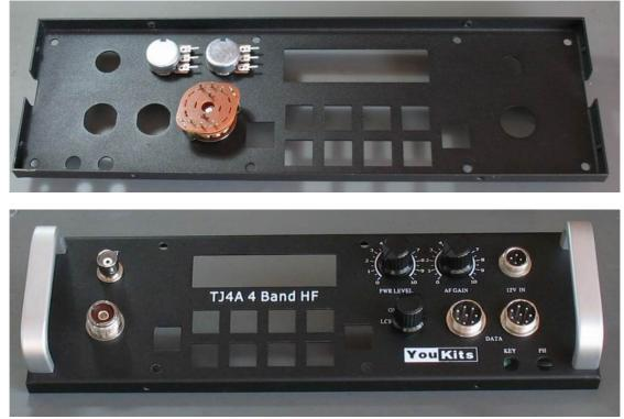
Do not use the long crews supplied with the handles. Find 4 shorter ones in the kit to fasten the handle to the front face. Remove the stopper of the pot with pliers. The power switch should be installed at a certain angle (See illustration).
