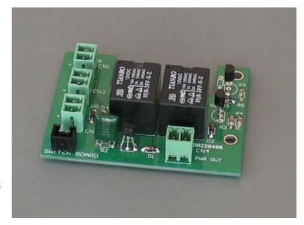
power, and **does not have current limiting device.** This connector only suits the battery **pack with charging management.** Insert a diode between the connector and the battery charging port, if necessary, to prevent the current flow back.
