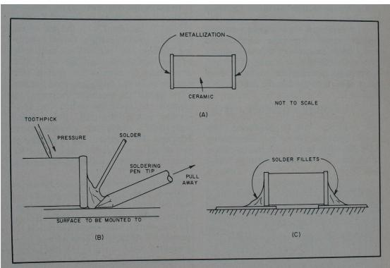
Fig. 24 — A typical chip capacitor is shown at A. The proper technique for holding and soldering the chip is shown at B. At C the final appearance of the capacitor in the circuit. Check for good solder flow, no metallization separation and no cracks or fractures in the ceramic.
