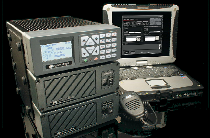
Barrett 2050 HF transceiver with 2023 modem, 2022 power supply and notebook PC running the Barrett 2020 Email fax and data system software
