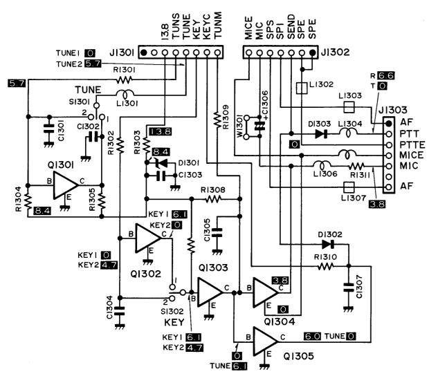
4.0 DC Voltage by 50K $\Omega$ -V multimeter
