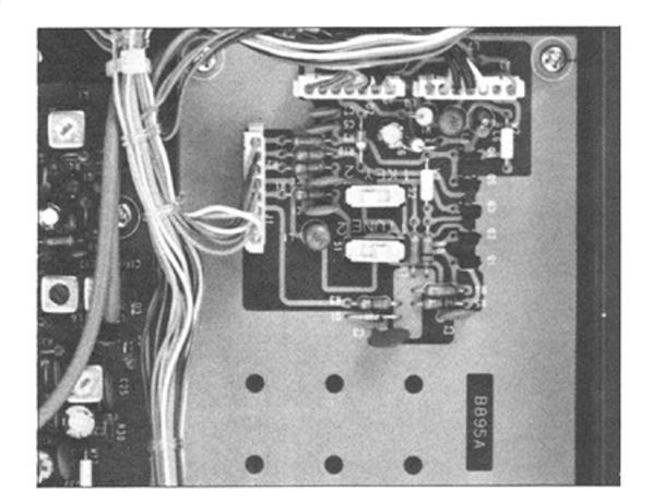
When S1 is set in the "2" position, the "START" terminal usually supplys about 8V DC through a 22K ohm resistor, and by pushing the TUNING SWITCH, the START terminal is grounded (0V) and sinks a current put out from the ANTENNA TUNER.
