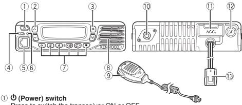
Press to switch the transceiver ON or OFF.
