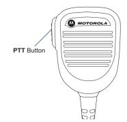
The microphone is activated when the **PTT** button is pressed.
