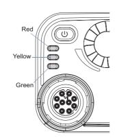
**Double blinking yellow** – Radio is no longer connected to the repeater while in Capacity Plus, all Capacity Plus channels are currently busy or in locked status.
