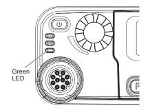
**NOTE:** The green LED lights up while the radio is transmitting and blinks rapidly when the radio is receiving a privacyenabled call.
