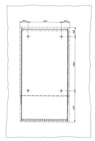
Free space for air circulation. Ambient temperature: Max. 40°C. Weight: T2130: 14 kg
