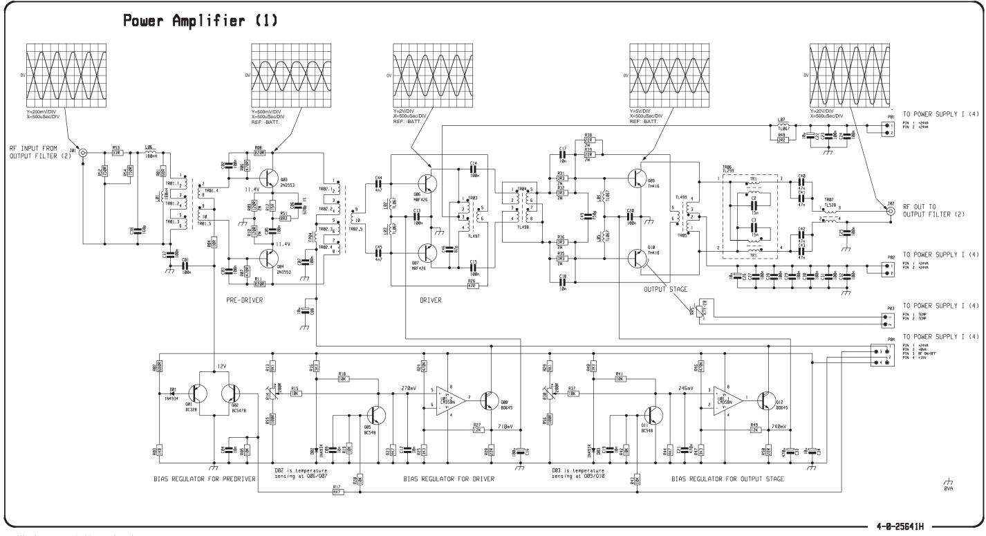
All voltages measured with transmitter in Service mode SP-29
