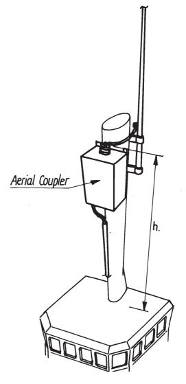
Example 4. AT2110 mounted on a sailing ship.
