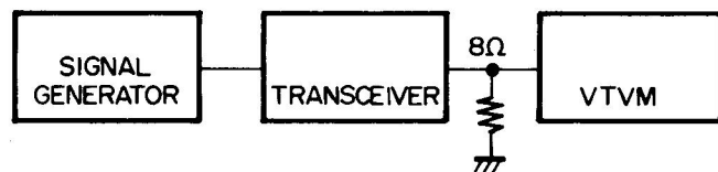
RX SENSITIVITY TEST SETUP
