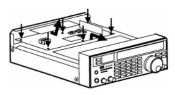
4 Locate position **MF1** on the I.F. PCB (refer to illustration). The position is currently unoccupied ready for the optional 500 Hz Collins mechanical filter. Use a desoldering pump to remove any excess solder from the respective pin positions. Insert the CW filter into the cleared holes of the PCB and securely solder its pins - don't overheat the filter!
