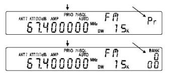
Use the *MAIN DIAL*, *SUB DIAL* or enter a three digit memory location via the numeric keypad. To transfer the data to PRIORITY press ENTER.
