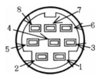
A standard 8-pin mini-din connector is used (which is widely available or the optional CR5000 tape lead may be used). The pin-outs for **ACC 1** are as follows:
