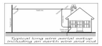
Keeping the aerial away from supports and building will reduce the loss of signal from the wire aerial and prevent unwanted noise from entering the aerial system.
