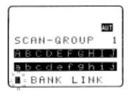
"BANK LINK" will be displayed on the bottom line of the LCD indicating that programming *is* possible.
