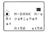
**2** Use the  $\Box$  key to move on to the resizing menu. The LCD will display the upper and lower case identifiers on the same line with the current default allocation of 50/50 channels per bank. Use the main dial or  $\Leftrightarrow$  keys to reallocate the channels in increments of 10 channels (60/40, 70/30, 80/20, 90/10, or 10/90, 20/80, 30/70, 40/60).
