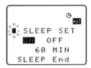
The AR8200 will automatically switch off after the programmed time has elapsed.
