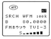
The selection of attenuator is held separately in each VFO, each memory channel and may also be toggled *during* search (in scan mode, the scanning process must be stopped in order to see which memory channel you are applying the attenuator to!).
