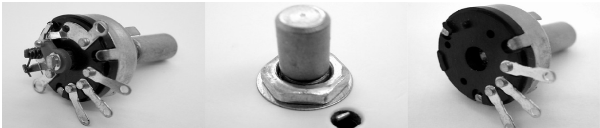
Fig.4. Volume control with on/off switch P2 (pot)
