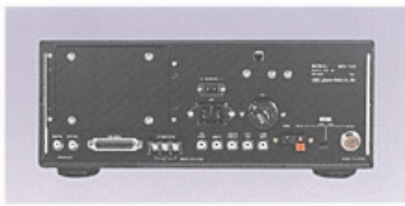
Rear panel of NRD-535 HF Receiver
