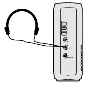
Because the radio is capable of receiving FM multiplex stereo, Stereo HEADPHONES Should be used. When listening to stereo FM, be sure that the FM: STEREO/MONO switch is set to the STEREO position.
