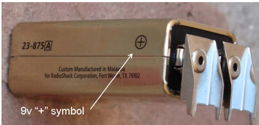
Figure 7. Find the 9v battery “+” symbol as shown above
