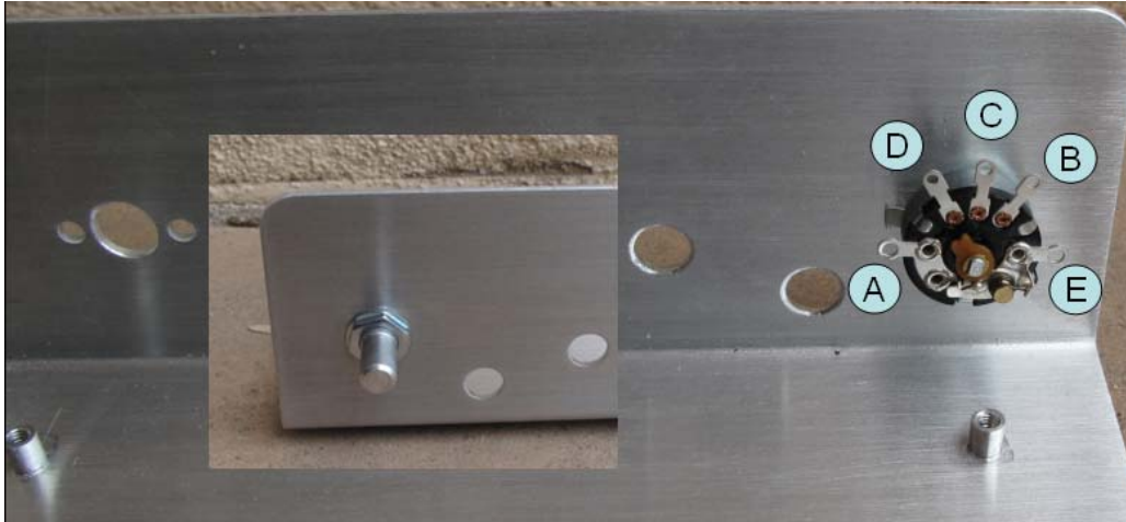
Figure 59. R6 (back view/front view) mounted to the front panel.
