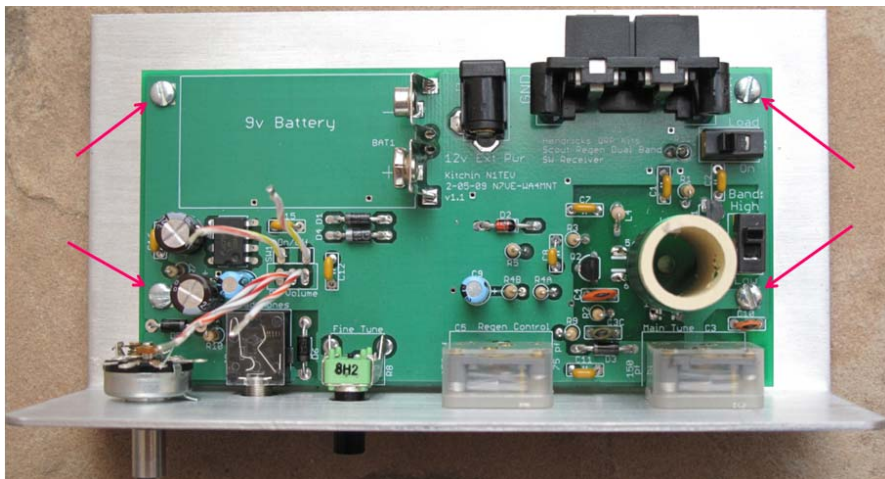
Figure 60. Mount the PC board with the four corner screws. Keep screws loose!
