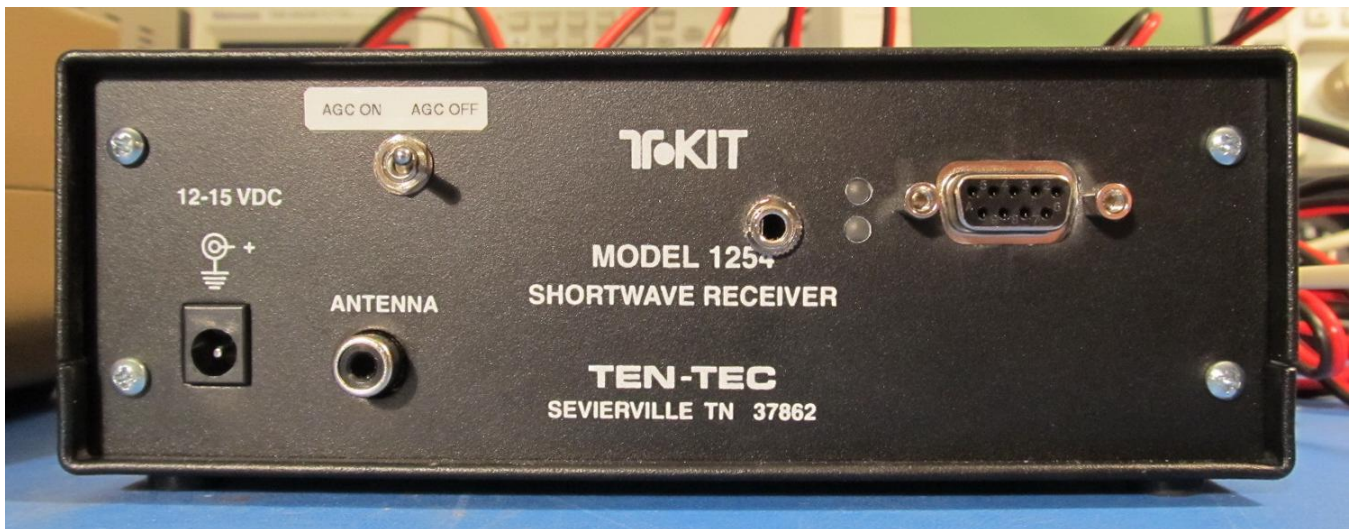
Figure 2 ~ Rear panel with new cutouts for the serial port interface and associated activity LEDs and auxiliary audio output jack on upper right side. The AGC on/off switch from the previous AGC modification is at top-left.
