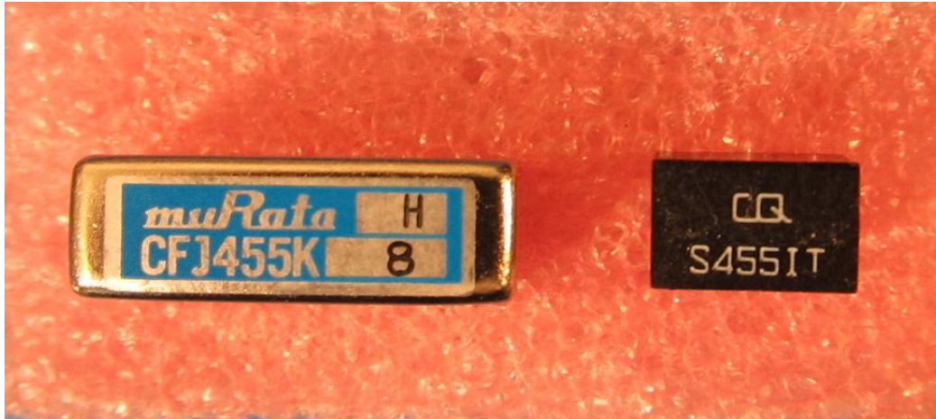
Figure 4 ~ New ceramic filter (left) has a nominal operating bandwidth of 1 kHz and original filter (right) has a 4 kHz bandwidth. The printed circuit board has solder pads for both configurations.
