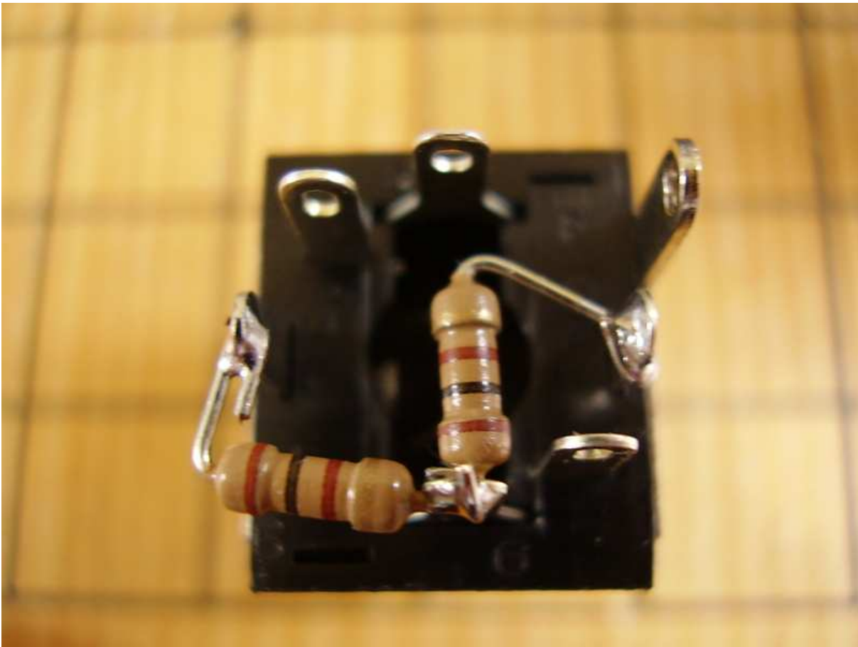
Figure 10.4: 100 Ohm Resistors Installed.
