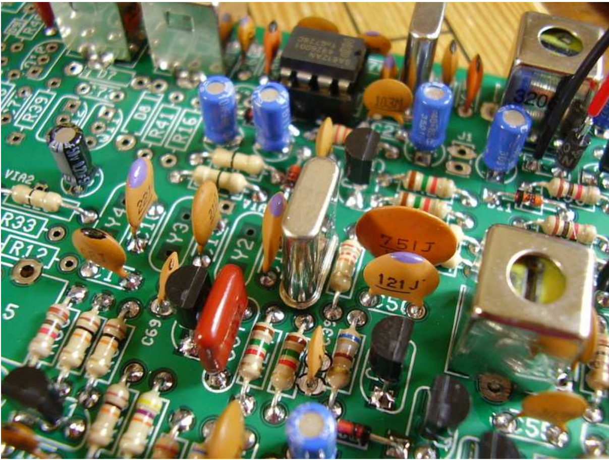
Figure 6.31: [4-33] [4-26] C17 68pF and Y1 14.31818MHz Crystal.
