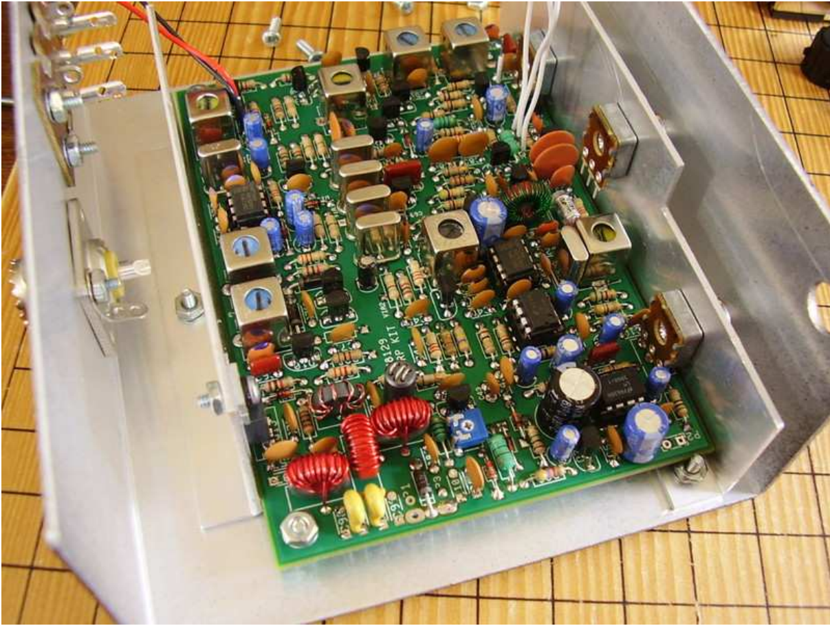
Figure 10.2: Board Installed in Center Shell.
