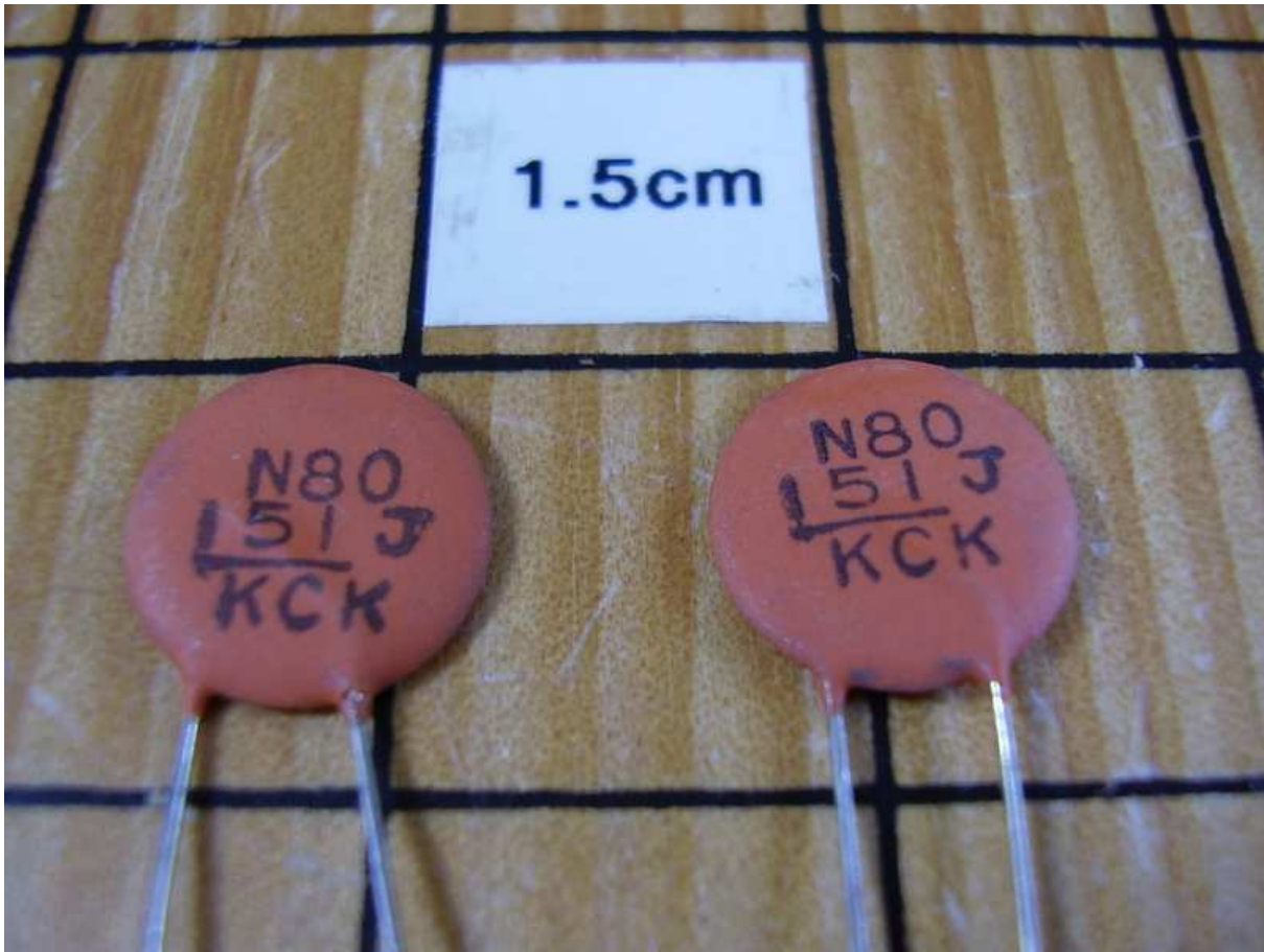
Figure 4.37: Photo of 150pF N80 Disc Caps.
