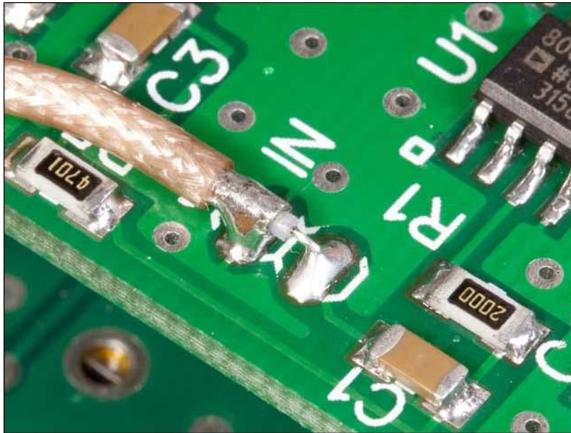
Figure 7: Coax attachment to Z10000 Buffer (Photo Courtesy of Roberto Barrios, EB4EQA)
