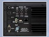
connecting appropriate cables to the ACC1 jack. No interface between rig and computer is necessary. Amp keying for QSK or non-QSK amps provided. Three SO-239 antenna connectors, two for transceive and a third for receive-only are on the opposite side of the heat sink.
