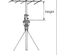
IMPOTANT: Keep the weight of the mounted antenna under 10 kg (22 lbs) for pole mounting.
