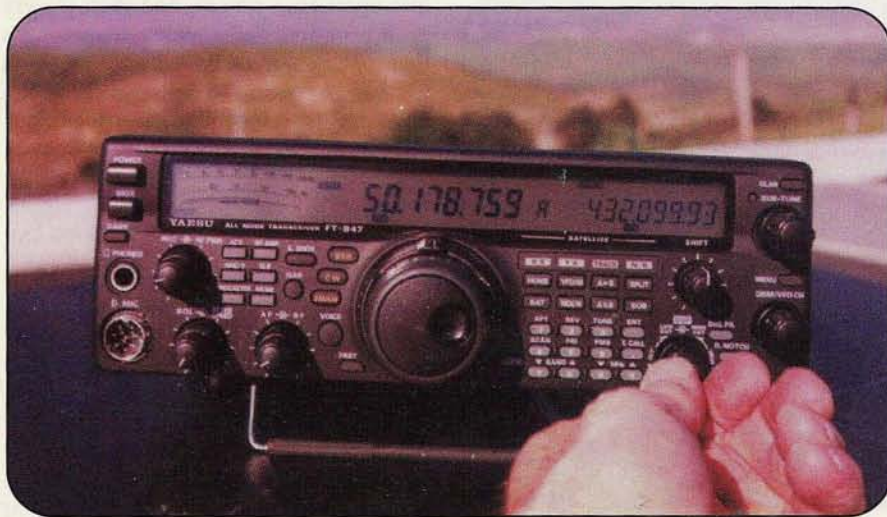
Photo E. The DSP (digital signal processing) filters improve signals on VHF at least as much as on HF. On 6 meters, DSP adjustments pulled in some 3,000-mile DX! (WB6NOA photo).
