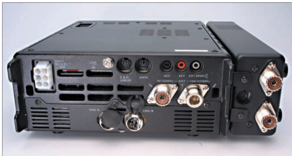
● Rear panel view of the FT-897. This transceiver provides portable 'Amateur Radio in one unit' from 1.8 to 430MHz, with many built-in features. You don't even have to carry a keyer for c.w. use...as it comes complete with a built-in version!
