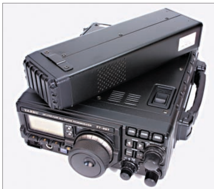
● The FT-897 with the optional automatic antenna tuning unit detached. The easy-carry 'rubberised' handle can be seen on the right.
