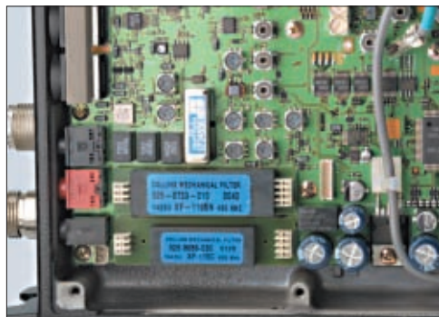
● Inside view of main chassis showing optional Collins filters fitted.
