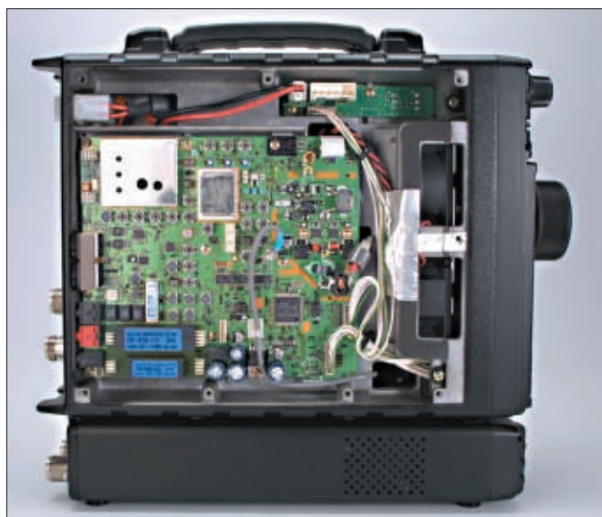
● Top inside view of transceiver showing auto antenna tuning unit.
