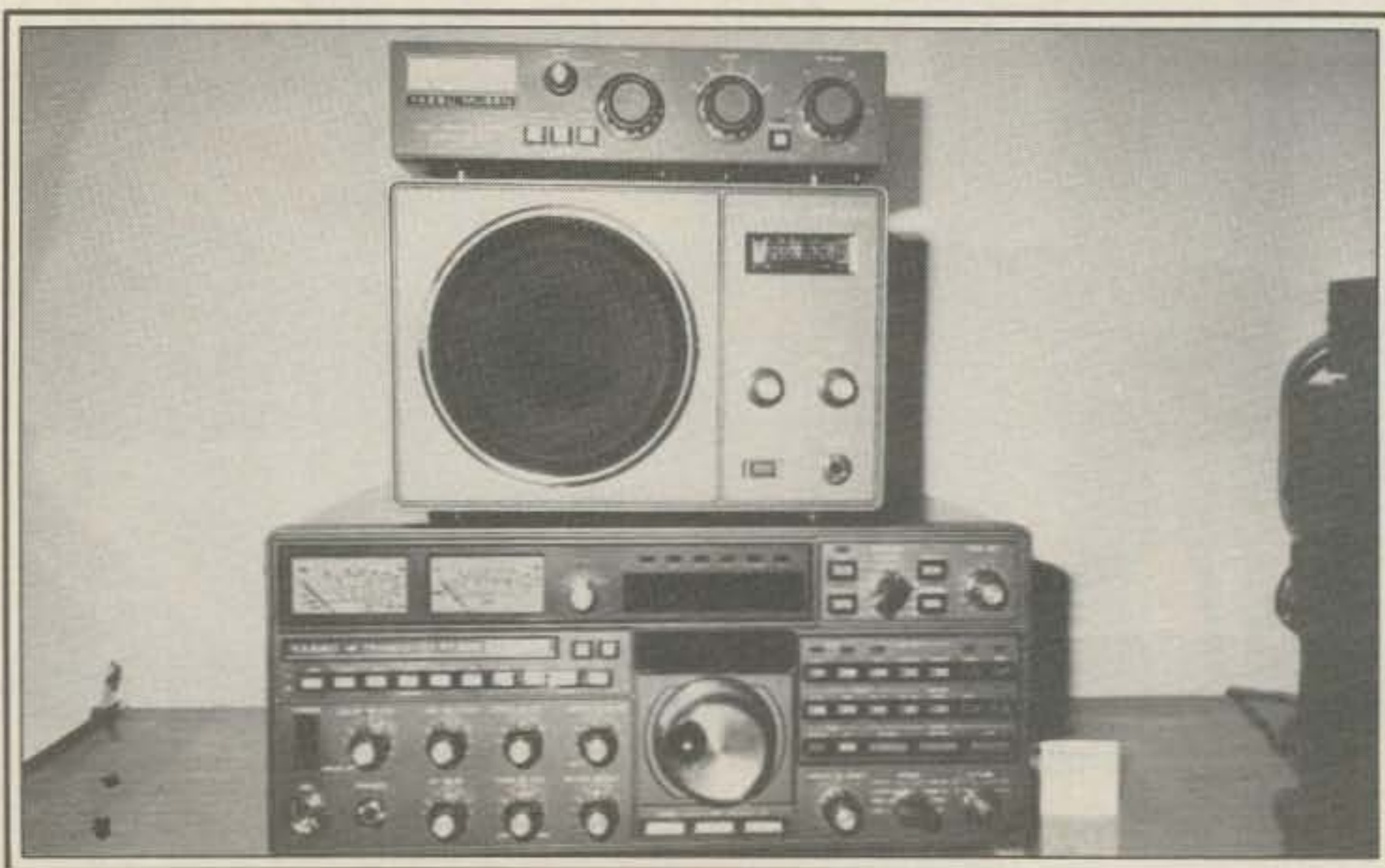
The FT-980 almost appears small here as it has stacked upon it the SP-980 optional speaker and a Yaesu FTV-707 transverter which can be used with the FT-980 for 2 meter coverage.
