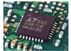
18 bit A/D converter for Narrow band SDR
