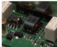
RF amp with the large size wide range transformer
