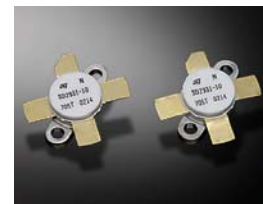
●200-Watt Version Utilizes Push-Pull SD2931 Devices
