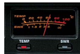
●Final Amplifier Temperature Display (MP/Contest Versions)
