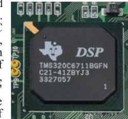
● 32-Bit High-Speed Floating-Point DSP
