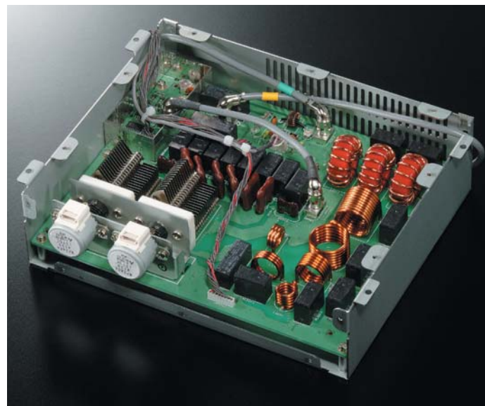
●Automatic, High-Speed 500-Watt-Capable Antenna Tuner
