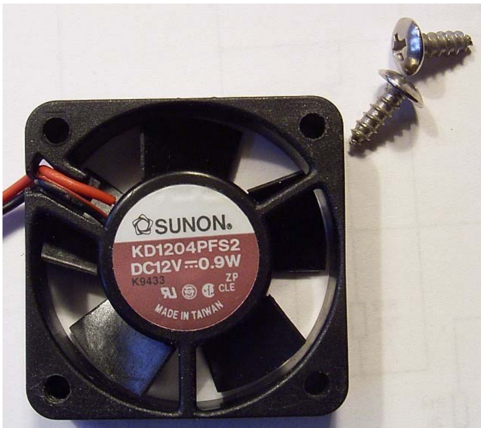
Fig 5. Fan with 2 x 3.5 mm screws
