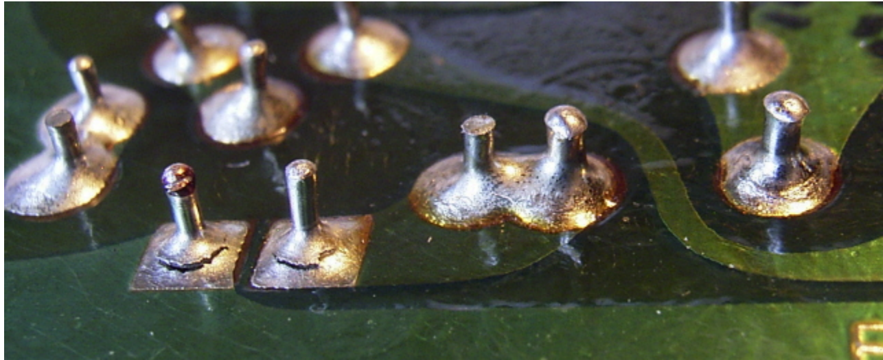
Fig 3. Close up photo showing cracked solder connections
