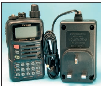
● Fig. 3: The rig has two main control knobs on the top of the unit - also showing the charging unit for size comparison - and these are ordinarily used to control the tuning and volume.
