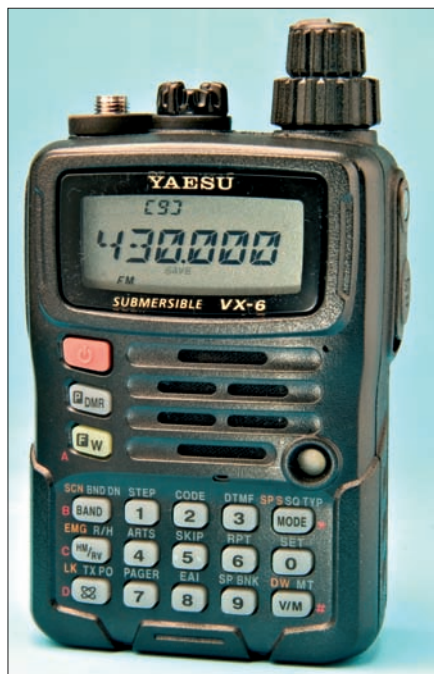
● Fig. 2: The Yaesu VX-6E although a dual-band transceiver, displays one band at a time (see text).
