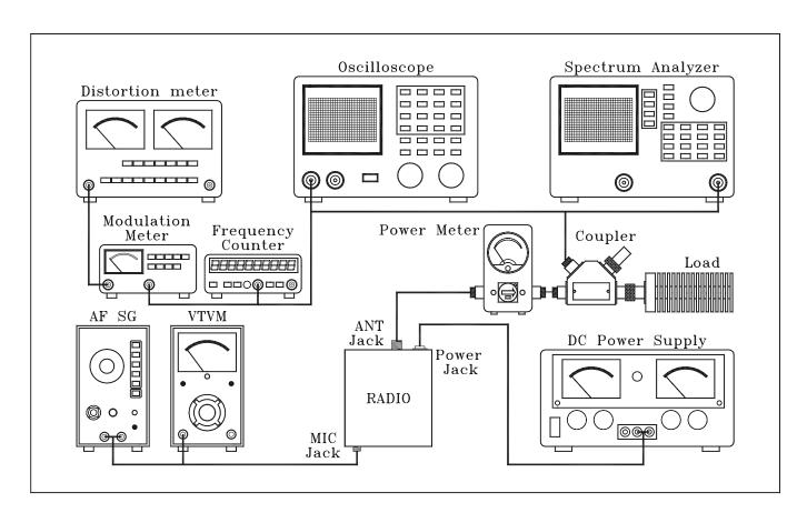
Figure 4.1.3 Receiver test setup
