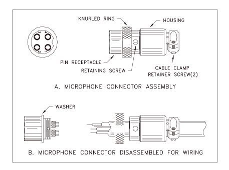
Fig. 2 Microphone plug wiring
