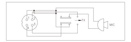
Fig. 1 Your transceiver microphone schematic.
