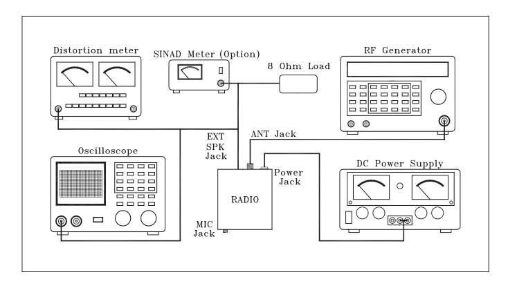
Figure 4.1.2 Transmitter test setup
