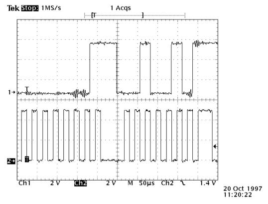
This picture shows the Data To Fader (DTF) waveform in comparison to the Clock. Note the first 8 clock pulses shift an address into the fader (in this case 00000001) and then the second 8 clock pulses
