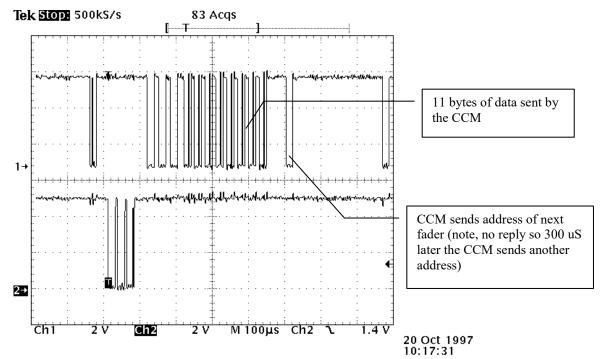
This drawing shows similar data transfer, but for a DC Master fader. Note the larger block of data sent to the fader by the CCM.
