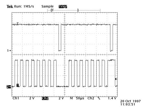
The picture above shows the Clock (lower) and Strobe (upper) lines as seen in a channel fader on P5025 pins 8 and 9. Note the first strobe pulse occurs while the clock line is low, this is an *Address Strobe*. The second strobe occurs while the clock line is high and this is a *Data Strobe*.
