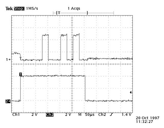
The picture above shows the fader emitting data (P5026 pin 19) referenced to the DEN signal (P5025 pin 14). Note the upper waveform shown at a non-logic voltage as the scan starts, this is characteristic of a High Impedance bus that is not being driven by anything. As soon as DEN turns on the bus assumes a correct voltage.
