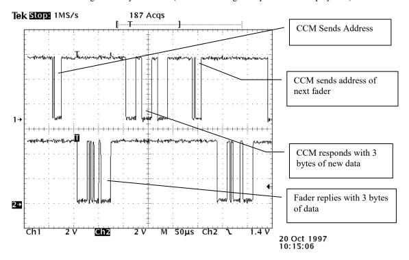
The picture above shows the waveforms seen on PCB7173, U14 pins 1 and 4. These are the individual transmit and receive lines before being combined into the bi-directional bus by U14 (on pins 6 and 7). The data shown is that of a channel fader (3 bytes sent and received).
