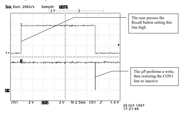
The picture above shows U3 pin 5, which goes high when the Recall button is pressed, then some tens of milliseconds later the  $\mu P$  performs a write (the narrow pulse on the lower trace) which clears the line back to a logic low.
